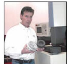
Tom Mullen, president of TNT EDM, holds an aluminum clutch housing on which internal and external splines are produced by EDM. The electrode in his other hand is one used to produce the internal splines. This long-running job is ideal for untended production on the automated CNC sinker cells.
