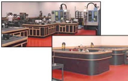
The motion of the robot is guarded by interlocking light curtains rather than by gates or enclosures. This arrangement makes the cells safe yet uncluttered. It is easy to scan the cell at a glance. With light curtains, there are fewer surfaces and moving parts to collect dirt or require maintenance. The carousel and robot can be reached easily for loading workpieces and/or electrodes.
