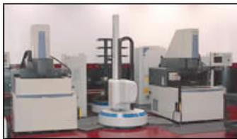
The left- and right-hand configuration of the sinker EDM units allows the machines to face the front while the robot is stationed in the middle.
