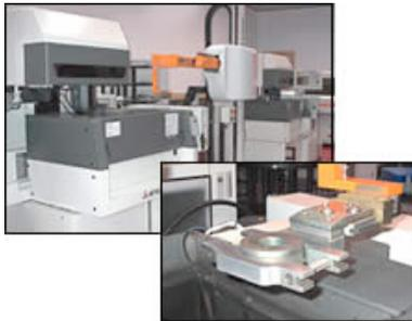
Like all of TNT's automated cells, this wire EDM cell features a robot and carousel between two machines. The robot loads either machine from the closest side, as shown directly above.
