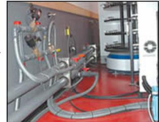
A look behind one of the automated cells reveals the tidy, accessible arrangement of utilities serving each machine tool. The large pipes running against the wall are connected to a centralized dielectric fluid system.
